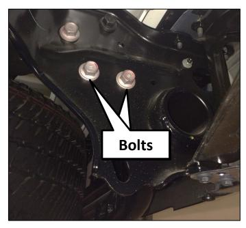
Install the bumper step by lining up the holes of the bumper step with the holes in the truck. Then reinstall the factory bolts that were removed in step one. Fully tighten the hardware.
